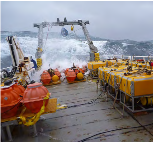
Ocean bottom seismometers waiting to be deployed during the Cascadia Initiative. Emilie Hooft, CC BY-ND
