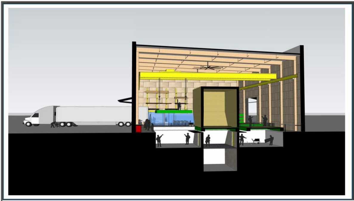
Figure 3 - Cross section of schematic design, through acoustics chamber
